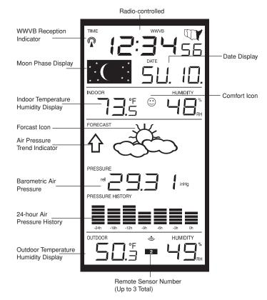
B. There are many different modes the indoor weather station can be set to. The LCD shown is the normal operating mode, and your actual data shown will be different based on your local settings and conditions.
